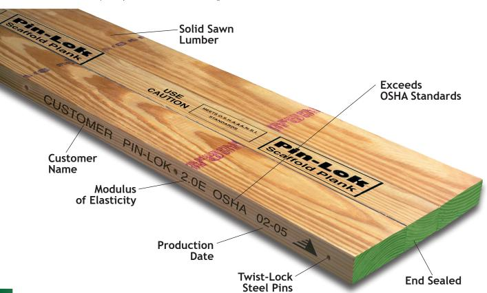
Twist-lock steel pins located every 22 inches are inserted through the wood members in a twist-lock operation. The holes drilled are actually slightly smaller than the grooved pins, so they must be twisted into place with high pressure. By joining the woods together with twisted steel pins in this fashion, the overall strength of the plank is greatly increased.
