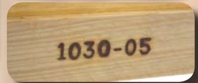
The optional branding unit can be used to automatically mark the plank with test information if the plank passes.
